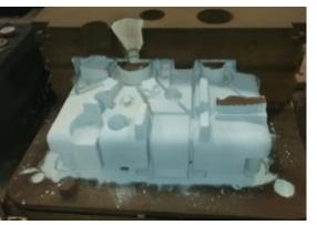
Figure 2: Partially assembled 3D printed mold
